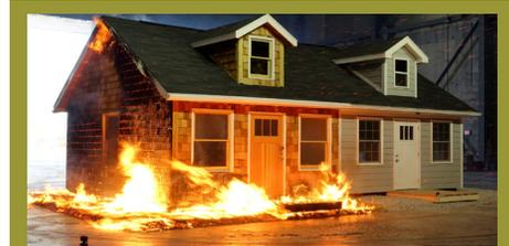
**Figure 1** – Creating and maintaining home ignition zones (defensible space) around your property are proven ways to reduce risks of property damage during a wildfire, as tests at the IBHS Research Center have shown.
